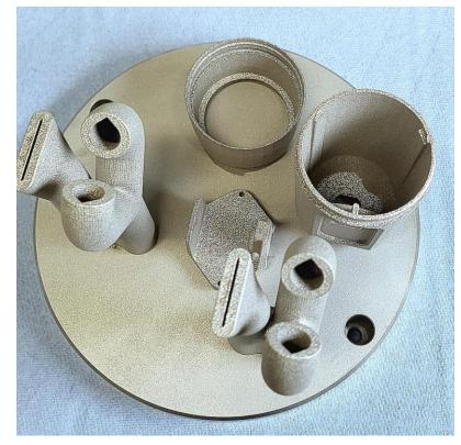
Combined nozzle for gas supply and crossjet for laser welding and parts for a rotary device for mounting on robot arm
